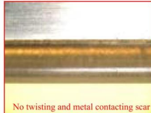
No twisting and metal contacting scar
